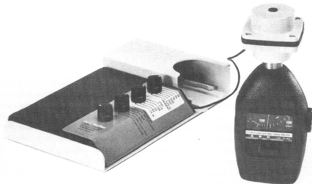
Figure 2-3. Typical calibration setup with a GR 1565-B Sound-Level Meter.
